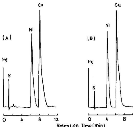
Fig. 6. HPLC separation of copper and nickel complexes of (A)  $H_2F_3A_2EMen$  and (B)  $H_2F_3AM_2EMen$ . Column, 250 mm  $\times$  4 mm I.D., Si 100 (5  $\mu$ m). (A) Eluent, chloroform-1,2-dichloroethane-*n*-hexane (15:3:82); flow-rate, 2.2  $cm^3\ min^{-1}$ ; detection, UV at 295 nm. (B) Eluent, chloroform-*n*-hexane (10:90); flow-rate, 2.0  $cm^3\ min^{-1}$ ; detection, UV at 300 nm.
