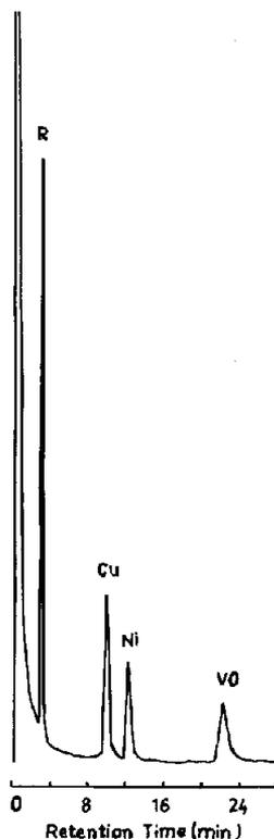
Fig. 4. GC separation of  $H_2A_2EMen$  and its Cu, Ni and VO complexes on a stainless-steel column (3 m  $\times$  3 mm I.D.) packed with 3% OV-17 on Chromosorb W HP (80–100 mesh). Column temperature, 250°C; injection port temperature, 270°C; nitrogen flow-rate, 30  $cm^3 min^{-1}$ .
