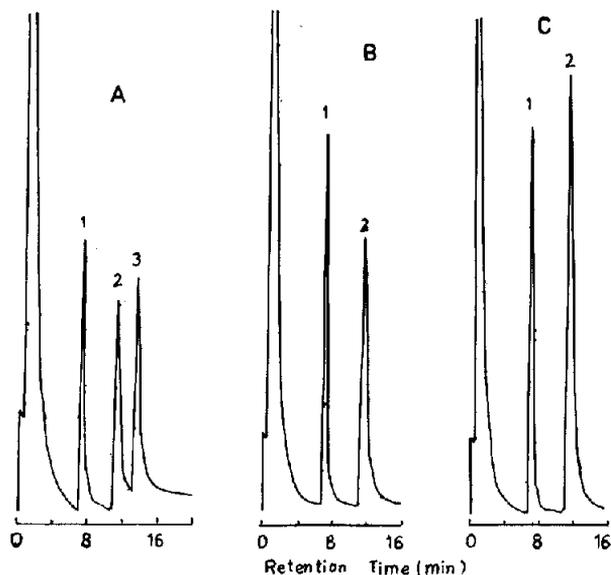
Fig. 5. Relative GC elution of (A) (1)  $F_3A_2EMeNi$ , (2)  $F_3AM_2EMeNi$  and (3)  $A_2EMeNi$ ; (B) (1)  $F_3A_2EMeCu$  and (2)  $A_2EMeCu$ ; (C) (1)  $F_3A_2EMeCu$  and (2)  $F_3AM_2EMeCu$ . Column, 3 m  $\times$  3 mm I.D., 3% OV-17 on Chromosorb W HP (80–100 mesh). Column temperature, 250°C; injection port temperature, 270°C; nitrogen flow-rate, 30 cm<sup>3</sup> min<sup>-1</sup>.
